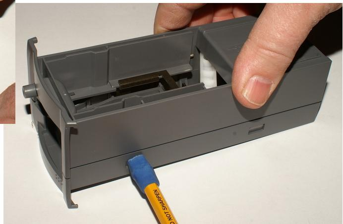
**2- Press in the four tabs (two on each side) and carefully pop the two halves apart.**
