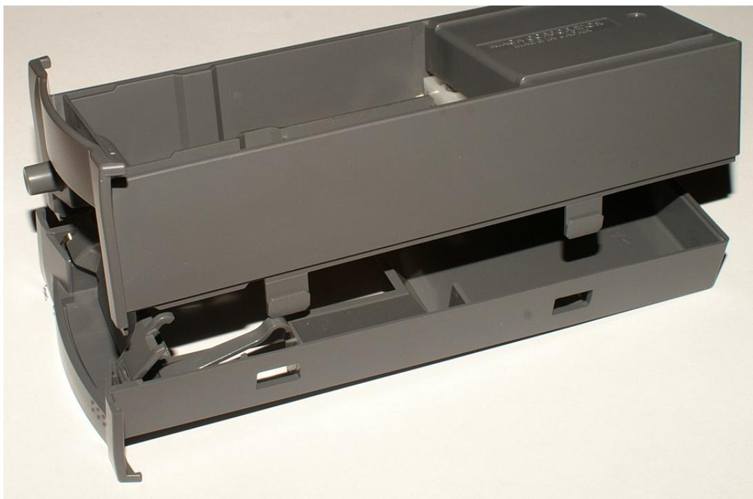
**3- Note spring in photo.** Do not remove spring or front access door shown. See spring in center below.
