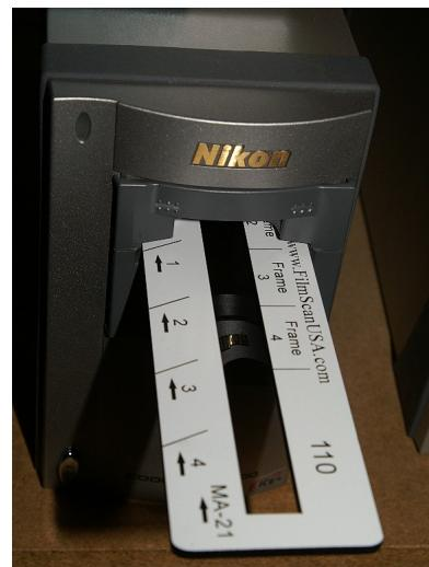
The MA-21-M modification allows our film holders to push in past the first frame to frames 2, 3, 4, etc.
