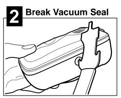
Insert sharp edge of hand tool into the vacuum-seal circle on bottom of camera to release pressure.
